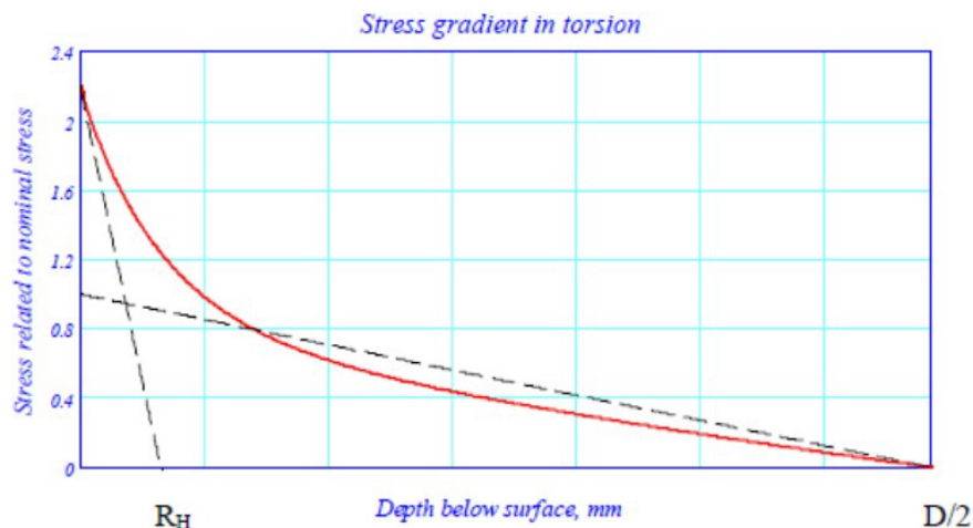
Figure G.3: Torsional SCF in the crankpin fillet as a function of depth. The corresponding SCF for the journal fillet can be found by replacing R_H with R_G and D with D_G
